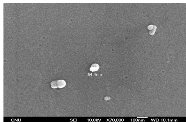
Fig. 1. SEM micrographs of SA–TSA nanoparticles produced with a SA:TSA mass ratio of 1:1.
